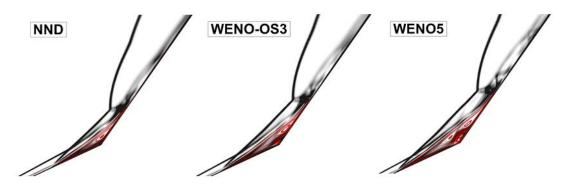
Fig. 3 Density gradient contours and separation region by different numerical schemes
