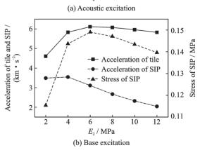
Fig. 7 Dynamic responses vs. elasticity modulus of SIP
