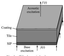
Fig. 1 Tile dynamic load sources
