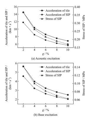
Fig. 5 Dynamic responses vs. structural damping coefficient
