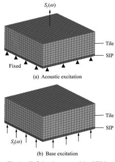
Fig. 4 3D finite element models of TPS
