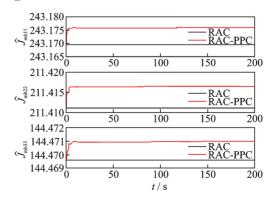
Fig.7 Time response of the estimated parameters of inertia
