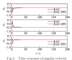
The steady control errors are presented in Table 3. As shown in Table 3, the attitude control errors under RAC-PPC are confined in the prescribed steady bounds. Furthermore, compared with RAC, RAC-PPC can achieve higher steady control precision.
