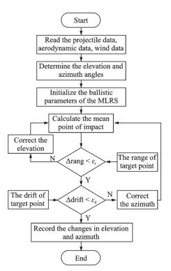
Fig.8 Flowchart of elevation and azimuth angle correction algorithm
