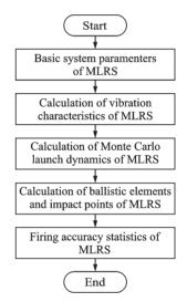
Fig. 3 Flowchart of launch and flight dynamics simulation system for MLRS
