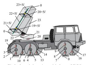
Fig.1 Launch dynamics model of a new MLRS
