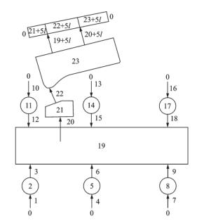
Fig.2 Topological diagram of a multiple launch rocket dynamics model
