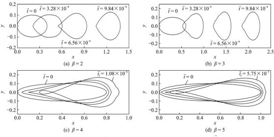
Fig.7 The evolution of intragranular microcracks with  $\chi = 0.54$  and  $\hat{h} = 5$
