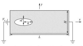
Fig.1 An intragranular microcrack in an interconnect line
