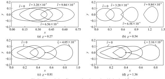
Fig.5 The evolution of intragranular microcracks with  $\beta = 2$  and  $\hat{h} = 5$
