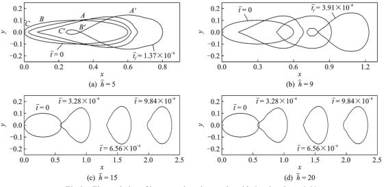
Fig.2 The evolution of intragranular microcracks with  $\beta = 3$  and  $\chi = 0.81$
