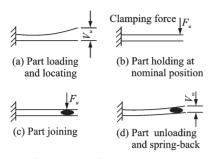
Fig.1 Compliant part assembly
