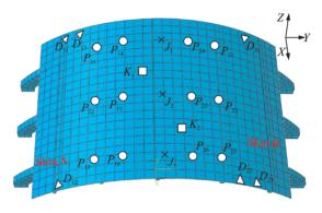
△ Deterministic locating point ○ Over-constrained locating point × Joining point □ Key product characteristic point Fig.10 FEA model of fuselage panel assembly
