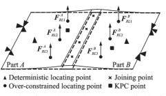
Fig.7 Clamping release at the over-constrained points
