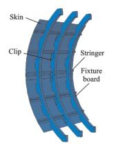
Fig.9 A typical 3D model of fuselage panel
