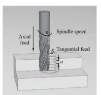
Fig.13 Schematic of helical milling process<sup>[69]</sup>
