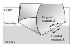
Fig.2 Schematic of drilling bi-material interface<sup>[21]</sup>
