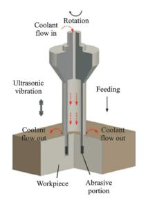
Fig.14 Illustration of ultrasonic assisted drilling<sup>[70]</sup>
