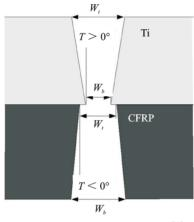
Fig.15 Example of kerf profile<sup>[79]</sup>
