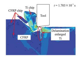
Fig.9 Chip formation process under the Ti→CFRP cutting sequence<sup>[43]</sup>
