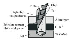
Fig. 3 Chip removal problems in drilling FRP/metal stacks<sup>[22]</sup>
