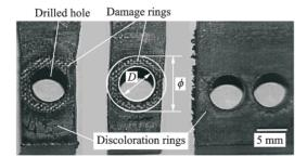
Fig.5 CFRP damage region at the CFRP/Ti interface<sup>[23]</sup>
