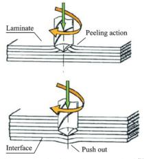
Fig.7 Delamination at the entry and exit<sup>[32]</sup>
