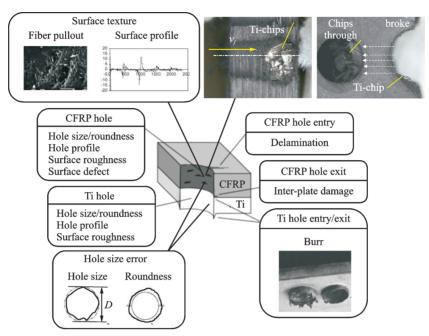
Fig.6 Hole quality features of FRP/metal stacks<sup>[8,30]</sup>
