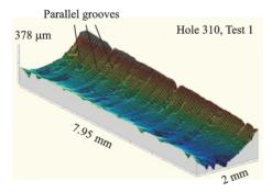
Fig.10 Topographic maps for the CFRP hole<sup>[6]</sup>
