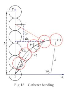
Considering the miniaturization and limited working space of the catheter, in this article, on the assumption that the catheter bends along an iso-curvature curve, the length of the central axis remains unchanged and skeleton balls are arrayed uniformly, let the bending angle is y, so
