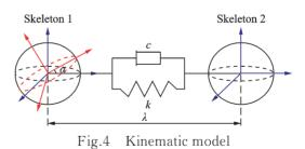
While an external force is applied to a skeleton ball, it can be resolved into  $F_a$  and  $F_t$ , where  $F_a$  is in the direction of the spring,  $F_t$  is the torsion force applied to the skeleton ball.
