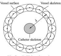
Fig.5 Collision detection
