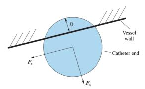
Fig.6 Feedback force calculating model
