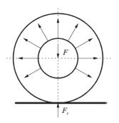
Fig.3 Load-carrying mechanism of NPMEW
