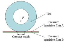
Fig.8 Mechanism of pressure sensitive film method
