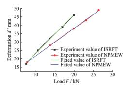
Fig.11 Load deformation curves of NPMEW and ISRFT
