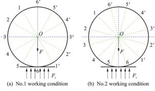
Fig.7 Two typical types of loading conditions for NPMEW
