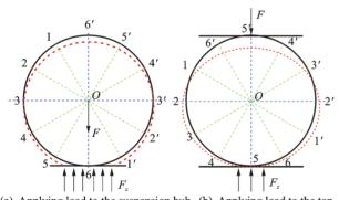
(a) Applying load to the suspension hub (b) Applying load to the top Fig.9 Load deformation behavior of NPMEW and flexible tire body at condition No.1
