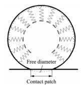
Fig.4 Deformation under vertical load
