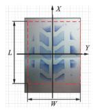
Fig.15 Contact pressure distribution coordinate system
