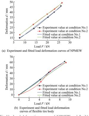
Fig.10 Load deformation curves of NPMEW and flexible tire body
