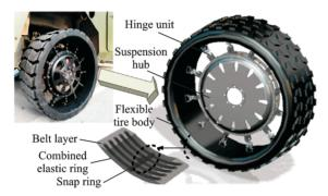
Fig.1 Non-pneumatic mechanical elastic wheel structure
