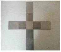
(b) Picture of cruciform specimen Fig.1 Shape of the cruciform specimen
