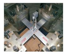
Fig.2 Establishment of the biaxial tensile test system
