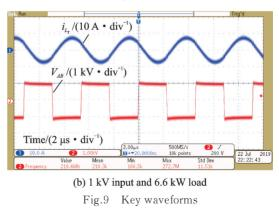
These waveforms show that the converter is able to work stably with the proposed inductor. The blue curve is the resonant current, and the red curve is the input voltage of the resonant tank. When the input voltage rises from 900 V to 1 kV, the switching frequency rises from 189 kHz to 210 kHz. From Fig. 9 (a), current waveform when  $f_s < f_r$  can be seen, and from Fig. 9(b), current waveform at the resonant frequency can be seen, which are consistent with the design before.
