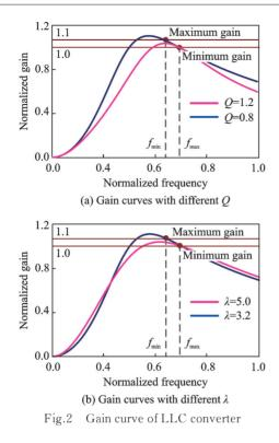
calculated as 0.71, however the DC gain cannot fulfill the requirement when the input voltage is 900 V either. Finally, Q=0.8 and  $\lambda = 3.2$  are chosen, since such parameters compromise between regulation capability<sup>[14]</sup> and the efficiency.
