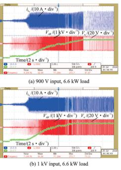
Fig.11 Soft start waveforms
