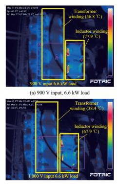
(b) 1 kV input, 6.6 kW load Fig.10 Thermal images
