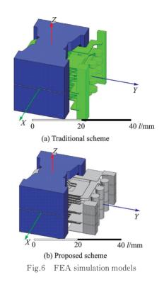
Table 1 shows the results of FEA simulation. The proposed scheme decreases the AC resistance by 24.15%, without changing the inductance. It is worth mentioning that the reduction of AC resistance means the reduction of copper loss, which contributes to the efficiency of the converter.
