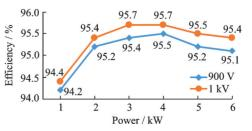
Fig.12 Efficiency curves under close-loop condition
