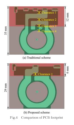
whole inductor reduce 17.14%. In addition, the terminal length decreases 50% from 12 mm to 6 mm, which will cause almost 50% terminal resistance reduction.
