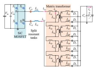
Fig.1 LLC converter with split resonant tanks
