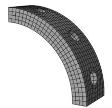
Fig.8 Geometry and finite element discretization of a quarter of the periodic part of the stent
