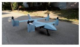
Fig.1 Tilt quad rotor with tilt-wing
