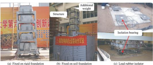
a) Fixed on rigid foundation (b) Fixed on soil foundation (c) Lead ru Fig.10 Tests of isolated structures on different foundations
