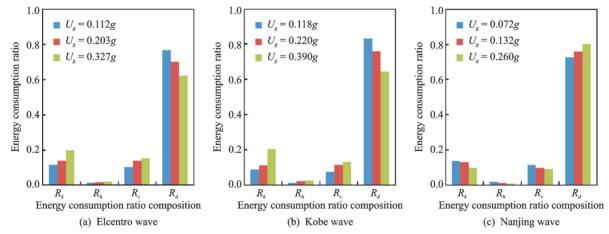
Fig.16 Ratio of energy dissipation of parts of isolated structure on softer interlayer soil foundation
