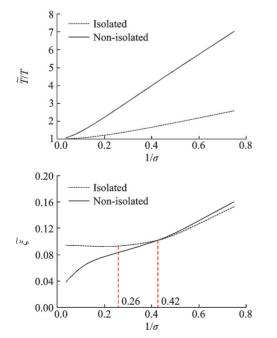
Fig.4 Natural period and damping of the SSI system as a function of wave parameter  $(1/\sigma)$
