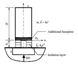
Fig.7 Calculation model of substructure method
