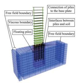
Fig.5 Numerical grid and model components in FLAC3D
