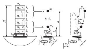
Fig.2 Simplified calculation mode of soil-base-isolatedstructure system
