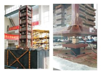
Fig.14 Test of high-rise isolated structure model on soil foundation
