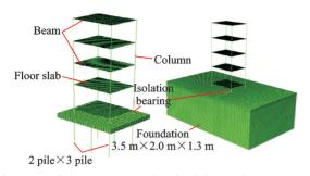
Fig.8 3D finite element model of soil-isolated structure system
