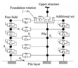
Fig.6 Calculating model of pile-soil-isloated structure
