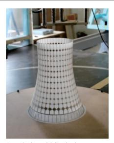
Fig.7 Aero-elastic model for simultaneous pressure and vibration measurement
