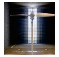
Fig.2 NREL Phase VI wind turbine in wind tunnel experiment
