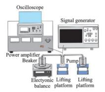
Fig.8 Experimental schematic of flow rate measurement
