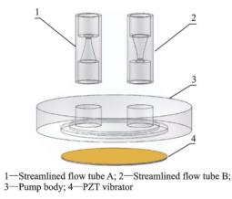
Fig.2 Exploded view of the streamlined pump
