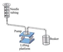
Fig.9 Experimental schematic diagram of flow resistance measurement
