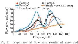
Fig.11 Experimental flow rate results of defonized water
