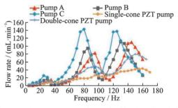
Fig.10 Flow rate comparison of white blood and deionized water in each pump
