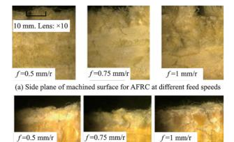
(b) Top plane of machined surface for AFRC at different feed speeds Fig.3 Delamination defects for AFRC for machining directions at 45°
