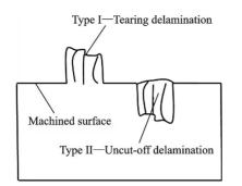
Fig.5 Types of delamination for machined surface
