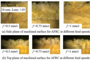
Fig.2 Delamination defects for AFRC for machining directions at 0°
