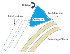
Fig.4 Schematic of the development of delamination
