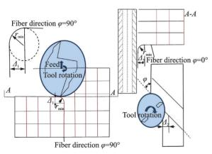
Fig.8 Bending of fibers in laminate and vertical planes
