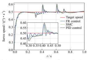
Fig.8 Servo speed control under multi-source disturbance
