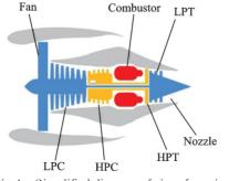
Fig.4 Simplified diagram of aircraft engine
