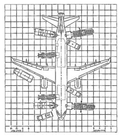
Fig.2 Servicing diagram of flight ground support vehicles
