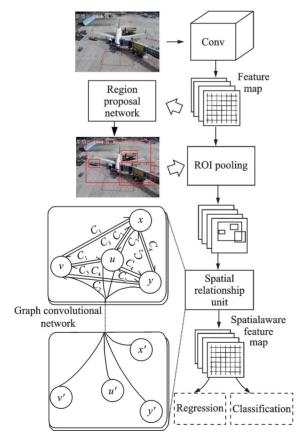
Fig.5 Architecture of the proposed SA-FRCNN
