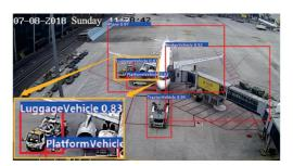
Fig.3 An actual example of Faster R-CNN in the apron
