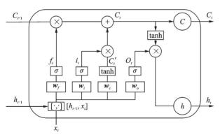
Fig.5 Structure of a basic LSTM cell
