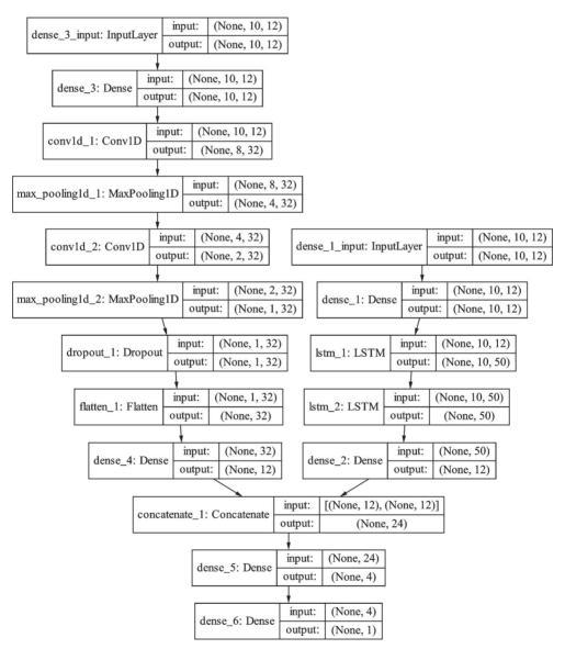
Fig.6 Structure and parameters of MICL model with 1-hour forecast period
