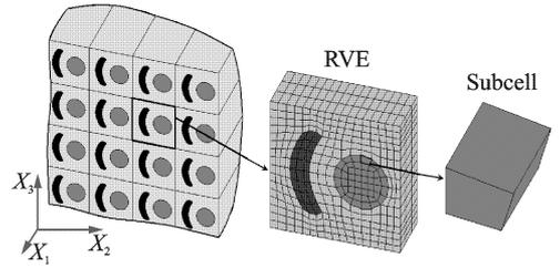
Fig. 1 RVE and subcells of fiber reinforced composites
