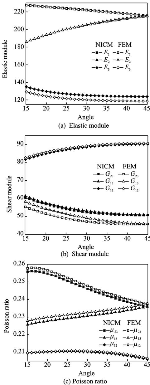
Fig. 8 Variation of mechanical properties with braided angle for braided composites
