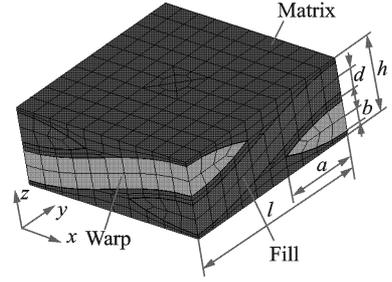
Fig. 3 Analytic model of woven fabric composites
