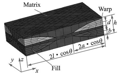
Fig. 5 Analytic model of braided fabric composites
