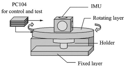
Fig. 1 Structure of rotating SINS
