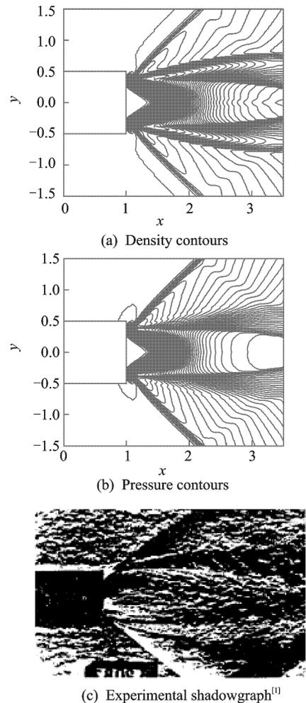
Fig. 3 Contours for Case 2 and experimental shadowgraph
