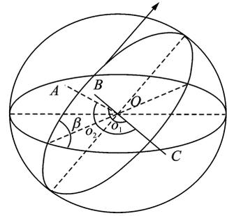
Fig. 5 Spatial geometrical relationship between location of user, reference point and geo-centre
