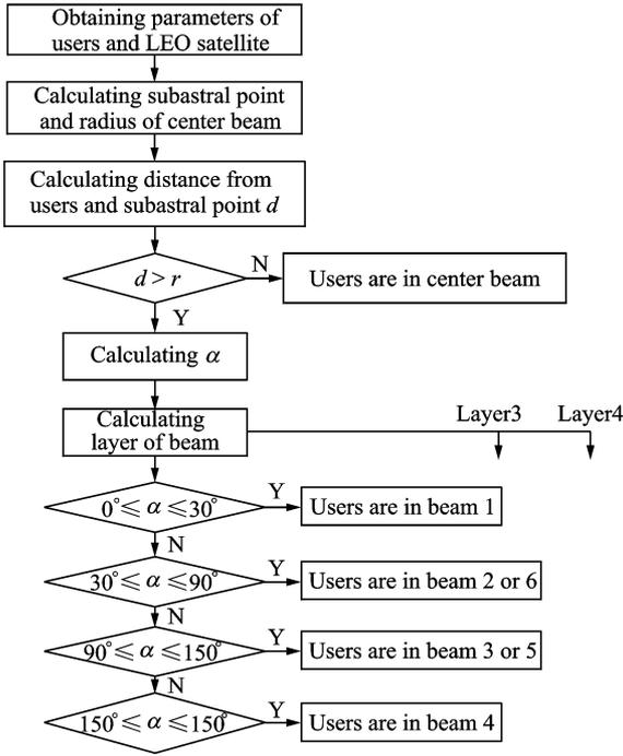
Fig. 6 Spot beam judgement of 2-D space process in system
