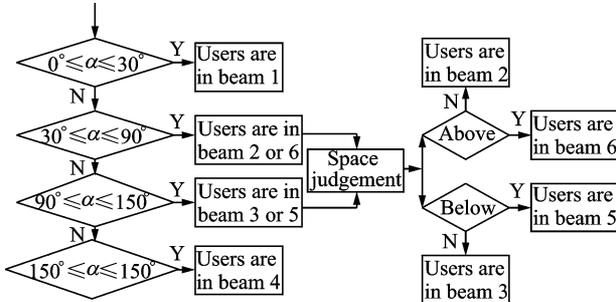
Fig. 7 Spot beam judgement of 3-D space process in system
