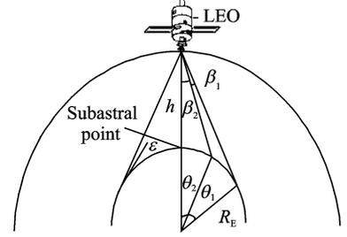
Fig. 1 Substellar point and spot beam
