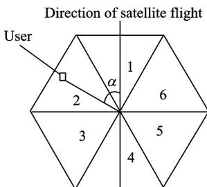
Fig. 2 Subastral beam coverage
