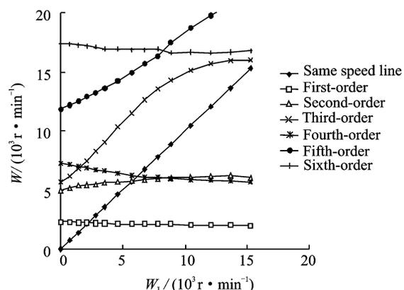
Fig. 4 Campbell graph excited by low-pressure rotor
