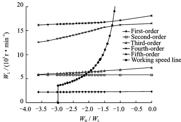
Fig. 8 Ray diagram excited by low-pressure rotor exciting
