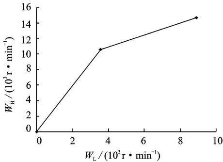
Fig. 3 Rotating speed relationship of dual-rotor aero-engine
