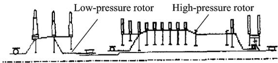
Fig. 1 Diagram of dual-rotor engine with five bearings
