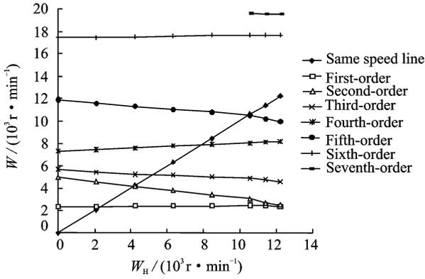
Fig. 5 Campbell graph excited by high-pressure rotor
