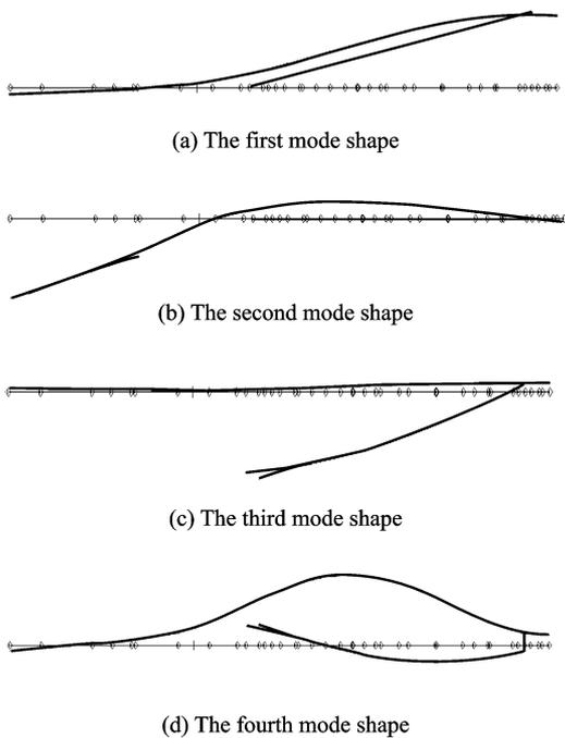
Fig. 6 The first four mode shapes excited by low-pressure rotor
