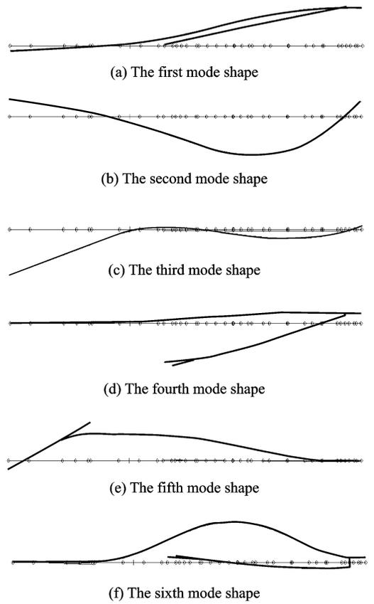
Fig. 7 The first six mode shapes excited by high-pressure rotor
