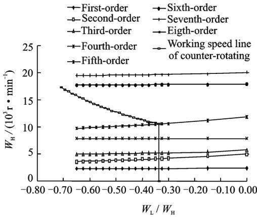
Fig. 9 Ray diagram excited by high-pressure rotor exciting
