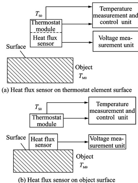
Fig. 2 Heat flux tactile sensor on different surfaces
