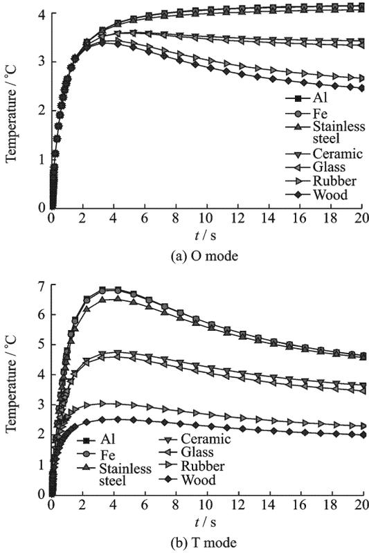
Fig. 5 Simulation results of different materials
