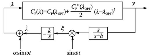
Fig. 6 Principle of single-parameter extremum seeking control
