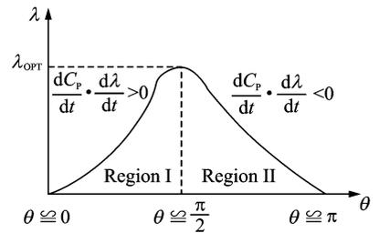
Fig. 7 Relationship between operation point and  $\theta$
