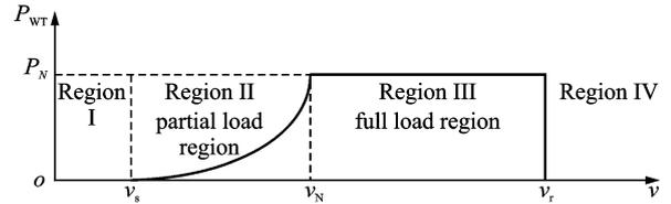
Fig. 1 Output power vs. wind speed characteristic
