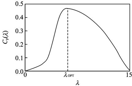
Fig. 2  $C_p$ - $\lambda$  curve of typical horizontal axis wind turbine
