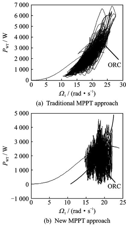
Fig. 10 Energy optimization curves based on two MPPT approaches
