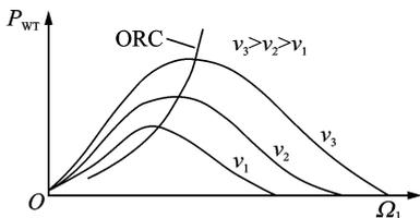
Fig. 3 Power characteristics parameterised by wind speed
