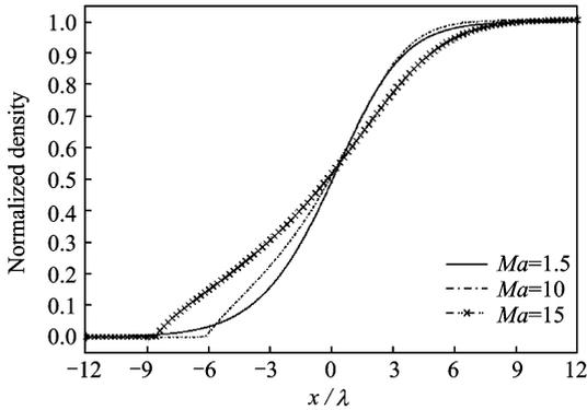
Fig. 6 Normalized density profiles at various Mach numbers with NCCR model
