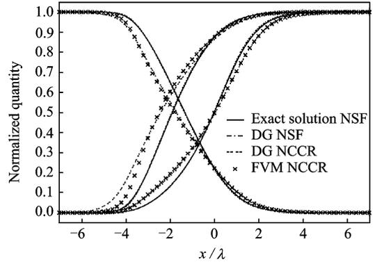
Fig. 3 Shock structure profiles at  $Ma=5$  with NSF and NCCR models
