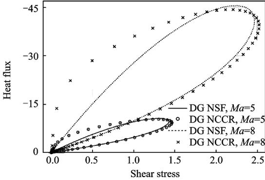
Fig. 5 Computational heat flux and shear stress at  $Ma=5$  and  $8$  with NSF and NCCR models
