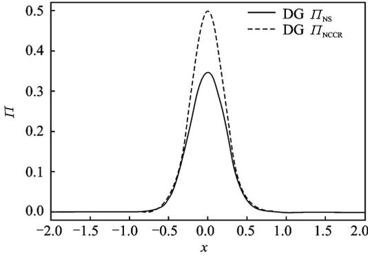
Fig. 2 Values of shear stress  $\Pi$  with NS and NCCR models
