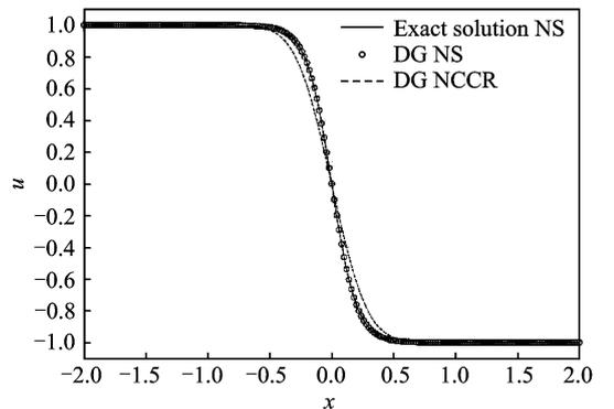
Fig. 1 Shock structure profiles of velocity with NS and NCCR models
