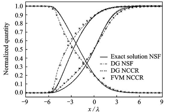
Fig. 4 Shock structure profiles at  $Ma=8$  with NSF and NCCR models
