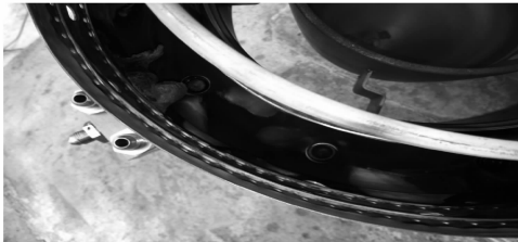
Fig. 7 Carbon deposition due to fuel spray
