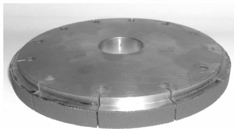
Fig. 1 Self-designed and prepared cBN wheel coated with polymer-based graphite lubricant
