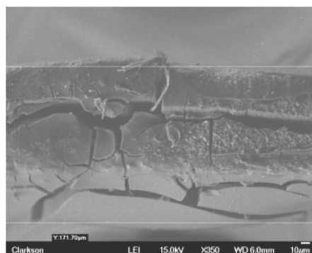
Fig. 6 Micrograph of anode thickness
