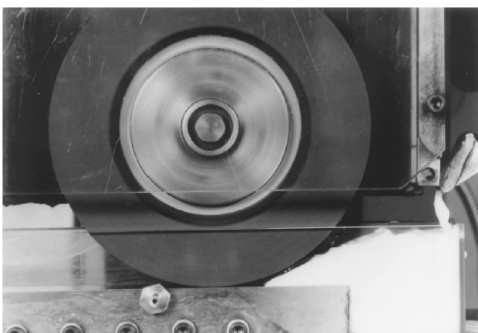
Fig. 14 Cutting fluid backing up due to boundary layer effects [83]
