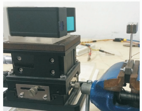
Fig. 9 Partial enlarged drawing of piezoelectric cantilever bimorph vibrator measured by laser head
