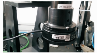
(f) Visual inspection components for testing welding result
