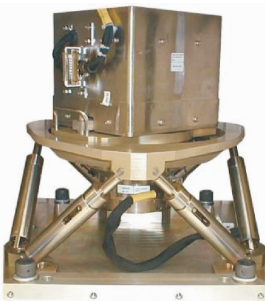
Fig. 1 Uniaxial rotation inertial navigation system [2]
