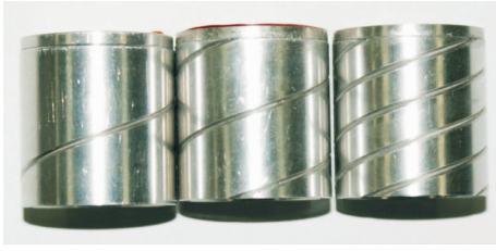
Fig. 8 Rotor structure with spiral slot
