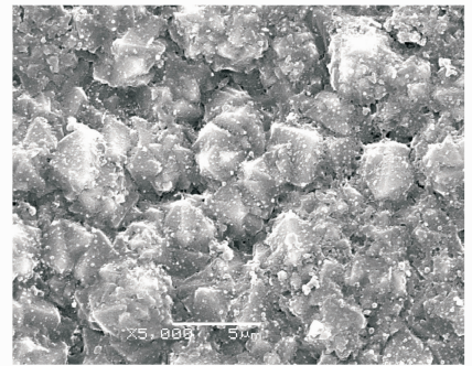
Fig. 7 SEM image of sapphire surface after lapping
