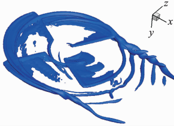
Fig. 8 Vorticity iso-surfaces for UH-60A rotor
