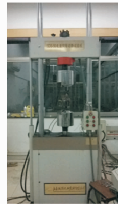
Fig. 1 SDS-50 electro hydraulic servo dynamic static and dynamic testing machine
