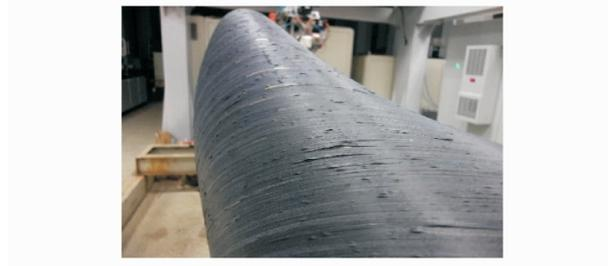
Fig. 4 Buckling defects in S-inlet AFP manufacturing
