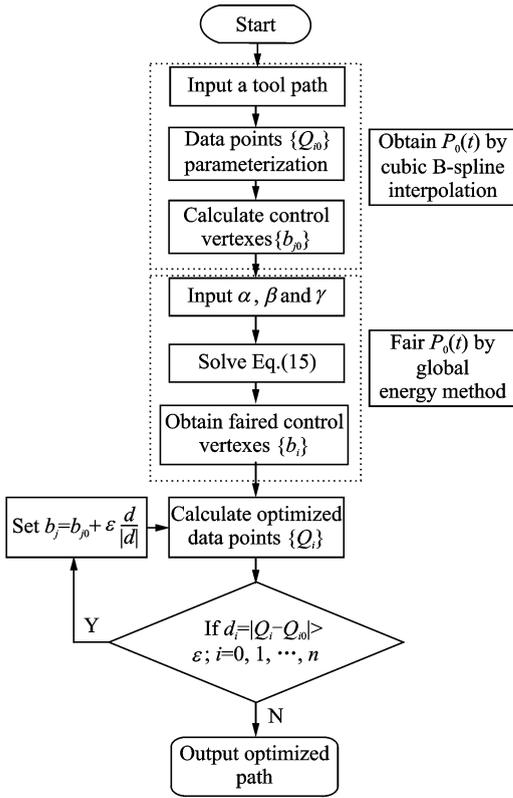
Fig. 5 Algorithm steps of global path faring for AFP
