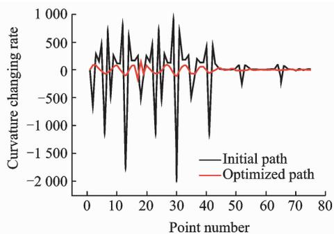
Fig. 8 Curvature change rate comparison between initial and optimized paths
