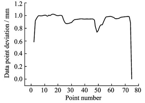
Fig. 6 Deviation of initial path after global faring treatment
