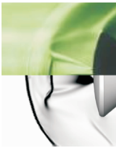
Fig. 4 Comparison between exp Schlieren picture (top) and CFD total density gradient contour (bottom)
