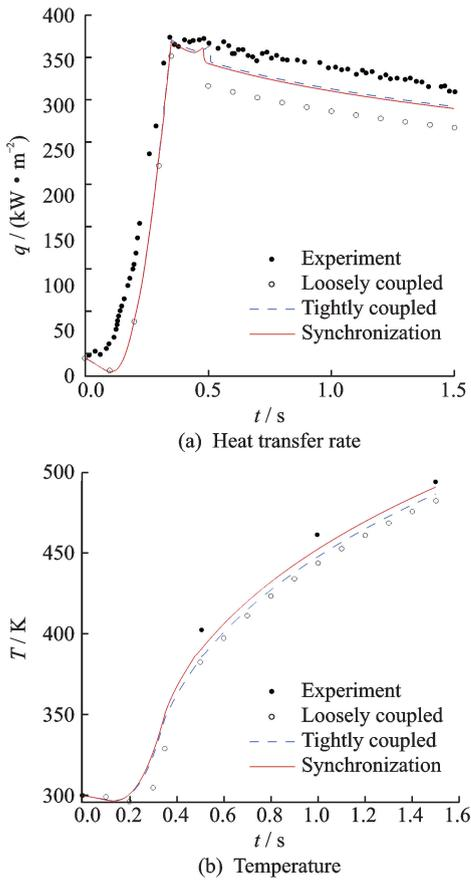
Fig. 13 Time history comparisons of heat transfer rates and temperatures at stagnation between the experiment, the loosely coupled method, the tightly coupled method, and the synchronization method
