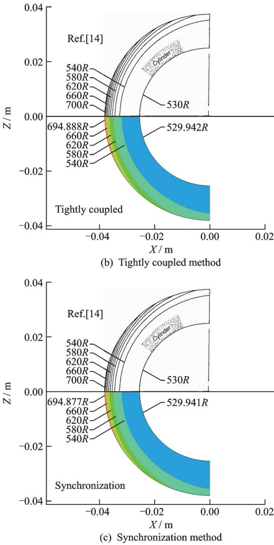
Fig. 6 Comparisons of predicted temperature contours at  $t = 2$  s of the loosely coupled method, the tightly coupled method and the synchronization method with the result in Ref. [14]
