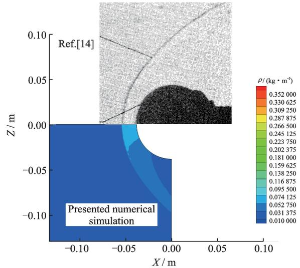
Fig. 5 Comparison of density contours between reference and present model for Mach-6.47 flow over a 3-in-diameter cylinder
