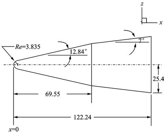
Fig. 8 Details of the profile of the model (mm)
