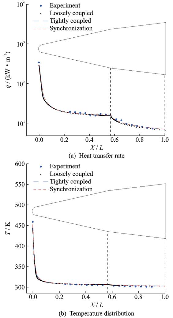
Fig. 10 Comparisons of the longitudinal heat transfer rates and temperature distributions at  $t=1.0$  s between the experiment, the loosely coupled method, the tightly coupled method, and the synchronization method
