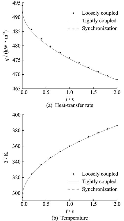
Fig. 7 Comparisons of heat-transfer rates and temperatures at stagnation between loosely coupled method, tightly coupled method, and synchronization method
