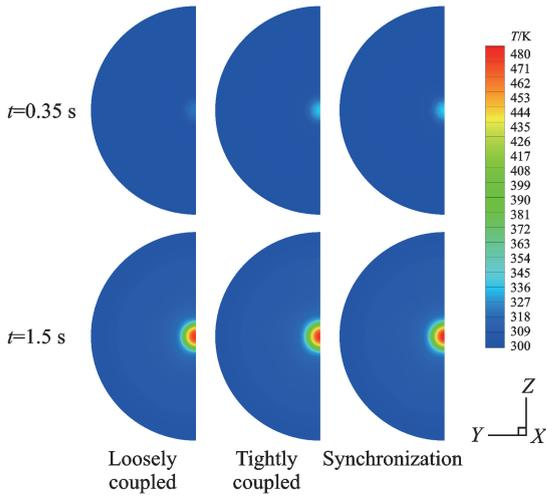
Fig. 11 Comparisons of temperature contours in solid domain at  $t=0.35$  s and  $t=1.5$  s between the loosely coupled method, the tightly coupled method, and the synchronization method
