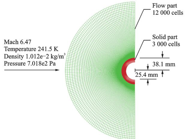
Fig. 3 Fluid-solid finite volume model for flow over a 76.2-mm-diameter cylinder
