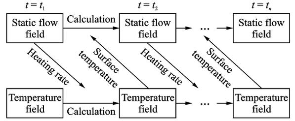
Fig. 1 Procedure for traditional coupling methods
