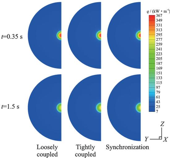
Fig. 12 Comparisons of surface heat flux contours at  $t=0.35$  s and  $t=1.5$  s between the loosely coupled method, the tightly coupled method, and the synchronization method
