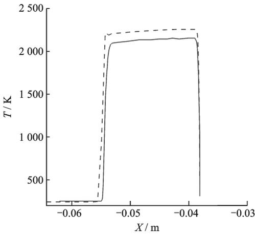
Fig. 4 Comparison of fluid temperature distributions between the reference and present model taken along the centerline of the initial flow
