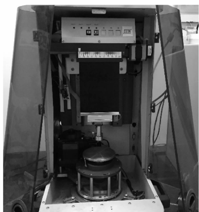
Fig. 6 Friction wear testing machine UMT-2
