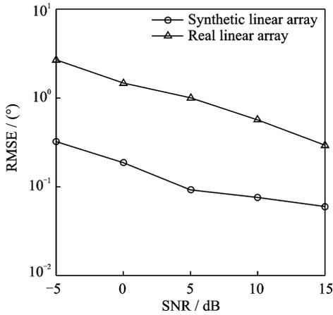
Fig. 4 Comparison of estimation performance with different arrays
