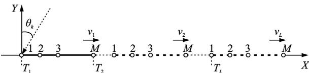
Fig. 1 Synthetic moving linear array model
