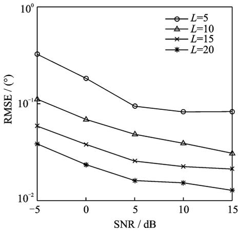
Fig. 5 DOA estimation performance with different  $L$
