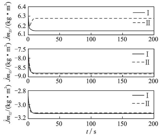
Fig. 8 Time response of the estimated parameters of the product of inertia
