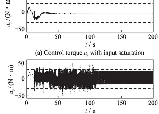
(a) Control torque  $u_y$  with input saturation
