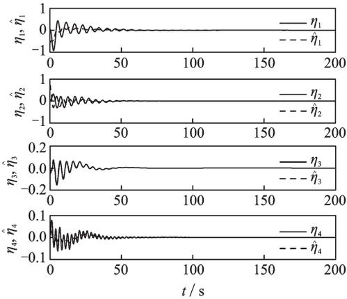
Fig. 5 Time response of vibration displacements and their estimates
