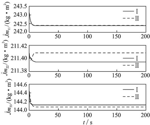
Fig. 7 Time response of the estimated parameters of inertia
