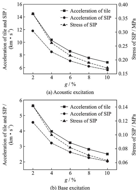
Fig. 5 Dynamic responses vs. structural damping coefficient
