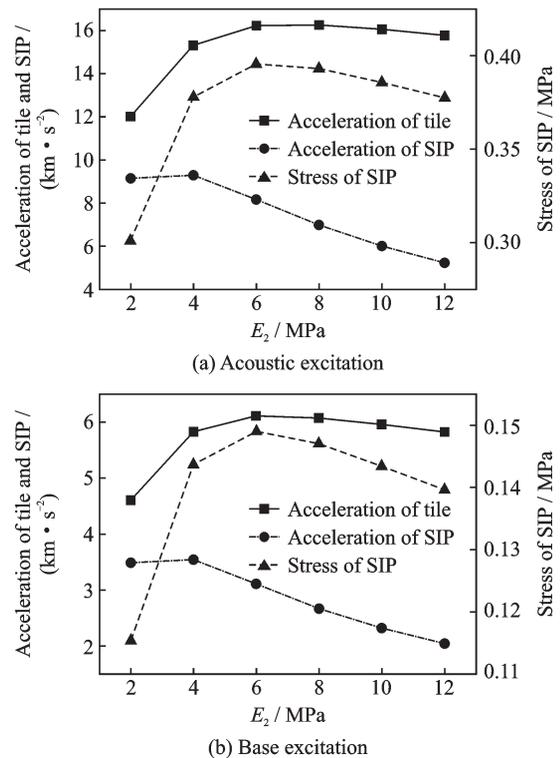
Fig. 7 Dynamic responses vs. elasticity modulus of SIP
