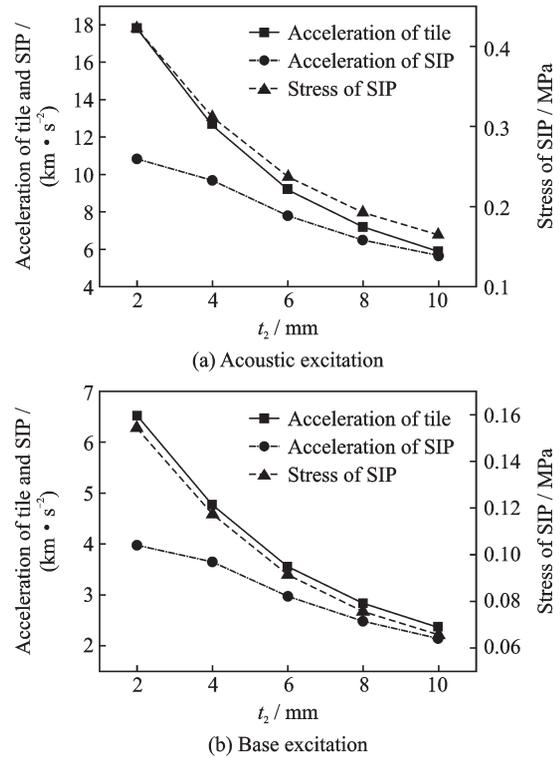
Fig. 6 Dynamic responses vs. thickness of SIP
