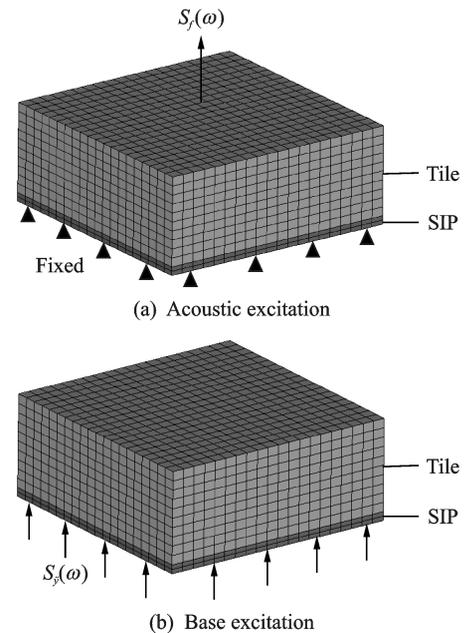
Fig. 4 3D finite element models of TPS
