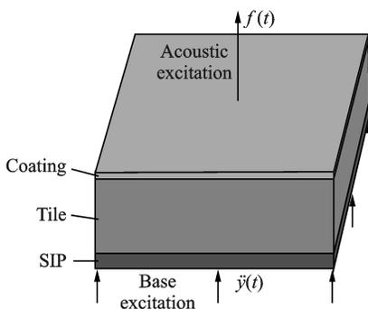
Fig. 1 Tile dynamic load sources
