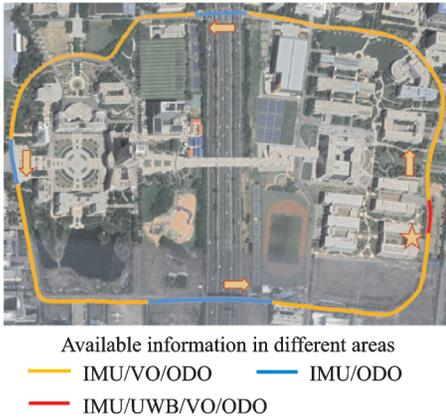
Fig.5 Field test in general road campus of NUAA
