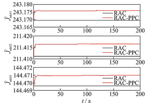
Fig.7 Time response of the estimated parameters of inertia
