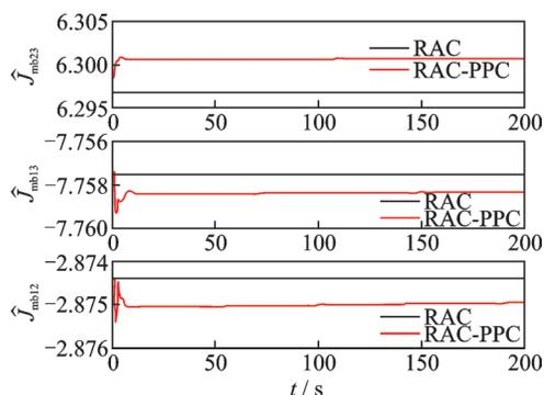
Fig. 8 Time response of the estimated parameters of the product of inertia
