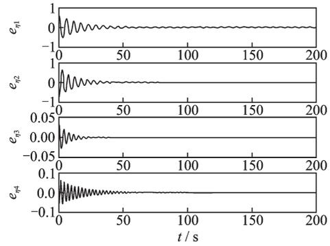
Fig.6 Time response of vibration estimate errors
